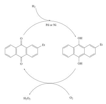
Fig. 15.8 The catalytic cycle used in the industrial manufacture of hydrogen peroxide;  $O_2$  is converted to  $H_2O_2$  during the oxidation of the organic alkylanthraquinol. The organic product is reduced by  $H_2$  in a Pd- or Ni-catalysed reaction. Such cycles are discussed in detail in *Chapter 26*.
