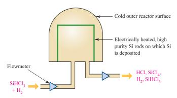
Fig. 27.8 Schematic representation of the CVD setup used to deposit high-purity silicon by thermal decomposition of SiHCl<sub>3</sub>.
