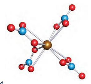
Fig. 8.6 The solid state structure (X-ray diffraction) of the  $[Zn(NO_3)_4]^{2-}$  anion in the salt  $[Ph_4As]_2[Zn(NO_3)_4]$ . Each  $[NO_3]^-$  ligand is coordinated to the Zn(II) centre through two O atoms, with one short (average 206 pm) and one long (average 258 pm) Zn—O interaction [C. Bellitto *et al.* (1976) *J. Chem. Soc., Dalton Trans.*, p. 989]. Colour code: Zn, brown; N, blue; O, red.
