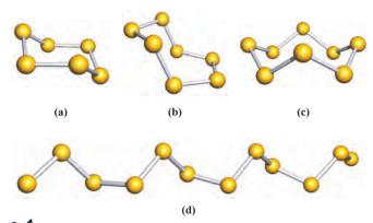
Fig. 15.6 Schematic representations of the structures of some allotropes of sulfur: (a)  $S_6$ , (b)  $S_7$ , (c)  $S_8$  and (d) *catena-S* $_{\infty}$  (the chain continues at each end).
