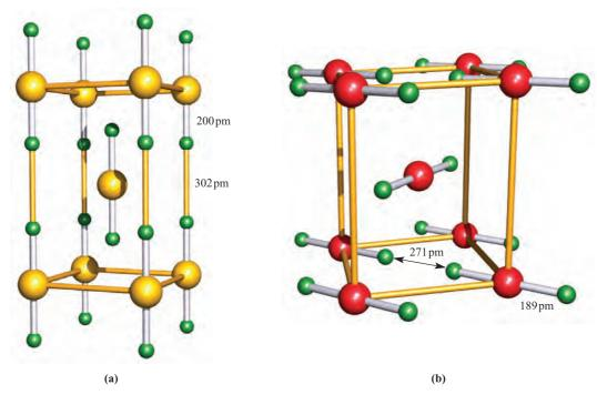
Fig. 17.4 Unit cells of (a) XeF<sub>2</sub> and (b) β-KrF<sub>2</sub> showing the arrangements and close proximity of molecular units. Colour code: Xe, yellow; Kr, red; F, green.
