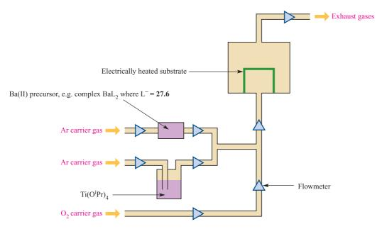
Fig. 27.13 Schematic representation of a CVD setup used for the deposition of the perovskite BaTiO<sub>3</sub>.
