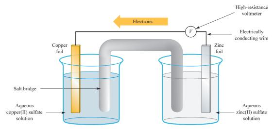
Fig. 7.1 A representation of the Daniell cell. In the left-hand cell,  $Cu^{2+}$  ions are reduced to copper metal, and in the right-hand cell, zinc metal is oxidized to  $Zn^{2+}$  ions. The cell diagram is written as:  $Zn(s)|Zn^{2+}(aq):Cu^{2+}(aq)|Cu(s)$ .
