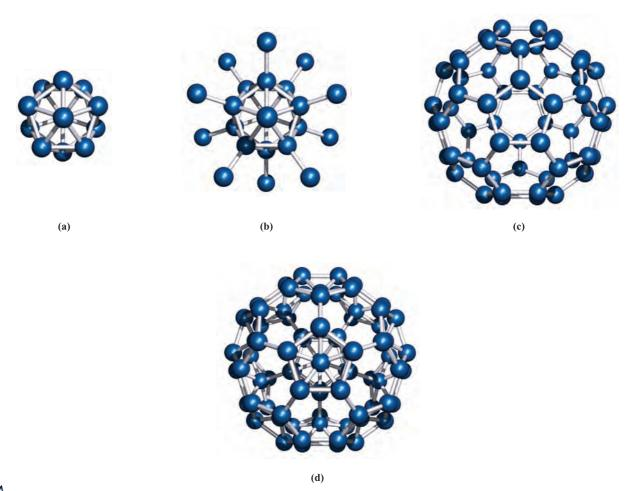
Fig. 12.6 The construction of the  $B_{84}$ -unit, the main building block of the infinite lattice of β-rhombohedral boron.
