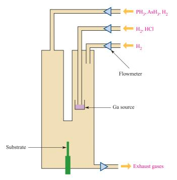
Fig. 27.11 Schematic representation of the CVD assembly used for the epitaxial growth of  $GaAs_{1-x}P_x$ ;  $H_2$  is the carrier gas.
