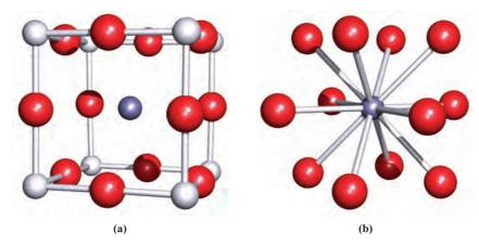
**Fig. 5.23** (a) One representation of a unit cell of perovskite (CaTiO<sub>3</sub>); (b) the Ca<sup>2+</sup> ion is 12-coordinate with respect to the  $O^{2-}$  ions. Colour code: Ca, purple; O, red; Ti, pale grey.
