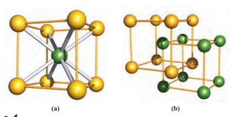
Fig. 5.16 (a) The unit cell of CsCl; Cs<sup>+</sup> ions are shown in yellow and Cl<sup>-</sup> in green, but the unit cell could also be drawn with the Cs<sup>+</sup> ion in the central site. The unit cell is defined by the yellow lines. (b) One way to describe the CsCl lattice is in terms of interpenetrating cubic units of Cs<sup>+</sup> and Cl<sup>-</sup> ions.
