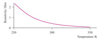
**Fig. 5.10** A semiconductor, such as germanium, is characterized by the fact that its electrical resistivity *decreases* as the temperature increases; thus, its electrical conductivity *increases* as the temperature increases.
