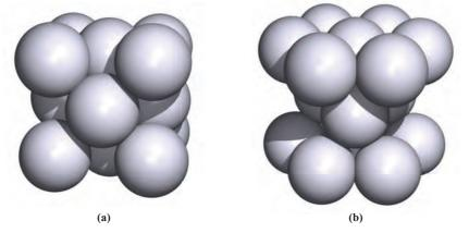
Fig. 5.4 Unit cells of (a) a cubic close-packed (face-centred cubic) lattice and (b) a hexagonal close-packed lattice.
