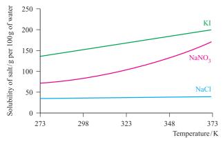
**Fig. 6.9** The temperature-dependence of the solubilities in water of potassium iodide and sodium nitrate. The solubility of sodium chloride is essentially temperature independent in the range 273–373 K.
