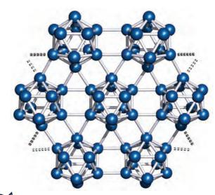
Fig. 12.5 Part of one layer of the infinite lattice of  $\alpha$ -rhombohedral boron, showing the  $B_{12}$ -icosahedral building blocks which are covalently linked to give a rigid, infinite lattice.
