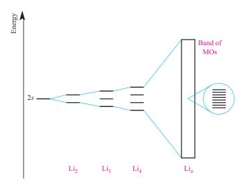
Fig. 5.11 The interaction of two 2s atomic orbitals in  $\text{Li}_2$  leads to the formation of two MOs. With three Li atoms, three MOs are formed, and so on. For  $\text{Li}_n$ , there are n molecular orbitals, but because the 2s atomic orbitals are all of the same energy, the energies of the MOs are very close together and constitute a *band* of orbitals.
