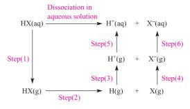
Fig. 6.3 The energetics of the dissociation of a hydrogen halide, HX (X = F, Cl, Br or I), in aqueous solution can be considered in terms of a cycle of steps. The significance of each step is discussed in the text.
