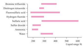
Fig. 8.2 Liquid ranges for water and selected non-aqueous solvents.
