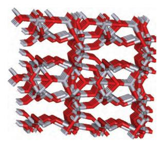
**Fig. 13.24** A 'stick' representation of part of the inorganic framework of the germanate  $[Ge_{10}O_{21}(OH)][N(CH_2CH_2NH_3)_3]$ . The  $[N(CH_2CH_2NH_3)_3]^{3+}$  cations are not shown but reside in the largest of the cavities in the network. The structure was determined by X-ray diffraction [L. Beitone *et al.* (2002) *Inorg. Chem.*, vol. 41, p. 3962]. Colour code: Ge, grey; O, red.
