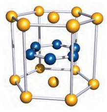
Fig. 27.7 A repeat unit in the solid state structure of MgB<sub>2</sub>. Colour code: Mg, yellow; B, blue.
