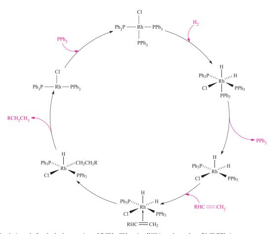
Fig. 26.5 Catalytic cycle for the hydrogenation of RCH=CH<sub>2</sub> using Wilkinson's catalyst, RhCl(PPh<sub>3</sub>)<sub>3</sub>.
