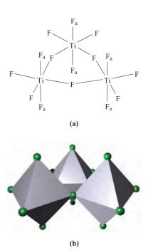
**Fig. 21.5** The solid state structure of TiF<sub>4</sub> consists of columnar stacks of corner-sharing octahedra. The building blocks are Ti<sub>3</sub>F<sub>15</sub>-units shown here in (a) schematic representation and (b) polyhedral representation; F atoms are shown in green. [Data: H. Bialowons *et al.* (1995) *Z. Anorg. Allg. Chem.*, vol. 621, p. 1227.]
