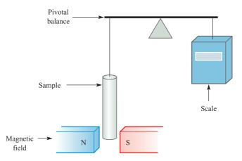
Fig. 20.21 Schematic representation of a Gouy balance.
