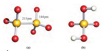
Fig. 15.17 (a) The structure of  $[S_2O_6]^{2-}$  showing the staggered conformation; from the salt  $[Zn\{H_2NNHC(O)Me\}_3][S_2O_6]\cdot 2.5H_2O$  [I.A. Krol *et al.* (1981) *Koord. Khim.*, vol. 7, p. 800]; (b) the  $C_2$  structure of gas-phase  $H_2SO_4$ . Colour code: S, yellow; O, red; H, white.
