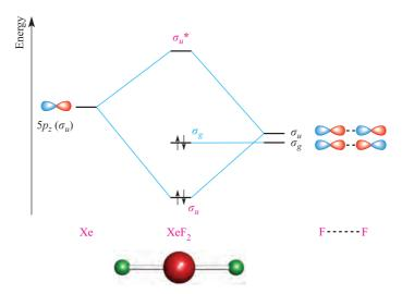
Fig. 4.30 A qualitative MO diagram for the formation of XeF<sub>2</sub> using a ligand group orbital approach and illustrating the 3c-2e bonding interaction.
