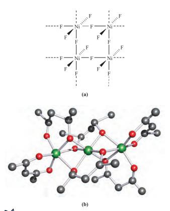
Fig. 21.27 (a) Representation of part of a layer of corner-sharing NiF<sub>6</sub> octahedra in K<sub>2</sub>NiF<sub>4</sub>. (b) The structure of [{Ni(acac)<sub>2</sub>}<sub>3</sub>] (X-ray diffraction) with H atoms omitted [G.J. Bullen *et al.* (1965) *Inorg. Chem.*, vol. 4, p. 456]. Colour code: Ni, green; C, grey; O, red.
