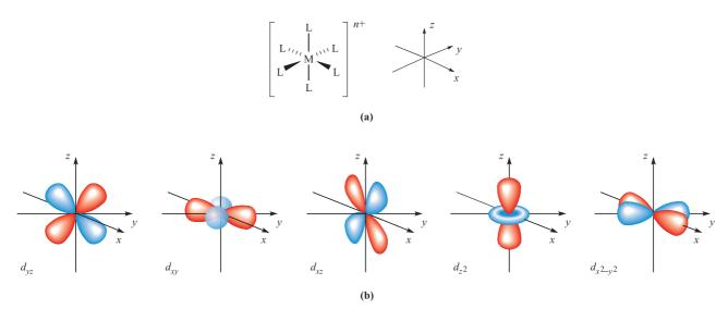
**Fig. 20.1** (a) The six M-L vectors of an octahedral complex  $[ML_6]^{n+}$  can be defined to lie along the x, y and z axes. (b) The five d orbitals; the  $d_{z^2}$  and  $d_{x^2-y^2}$  atomic orbitals point directly along the axes, but the  $d_{xy}$ ,  $d_{yz}$  and  $d_{xz}$  atomic orbitals point between them.
