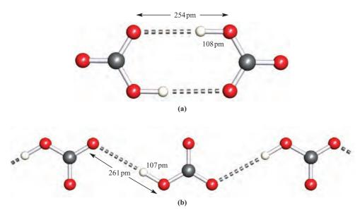
Fig. 10.7 In the solid state, hydrogen bonding results in anion association in NaHCO<sub>3</sub> and KHCO<sub>3</sub>, and the formation of (a) dimers in NaHCO<sub>3</sub> and (b) infinite chains in KHCO<sub>3</sub>. Colour code: C, grey; O, red; H, white.
