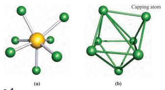
Fig. 17.6 (a) The structure of [XeF<sub>7</sub>]<sup>-</sup>, determined by X-ray diffraction for the caesium salt [A. Ellern *et al.* (1996) *Angew. Chem. Int. Ed. Engl.*, vol. 35, p. 1123]; (b) the capped octahedral arrangement of the F atoms in [XeF<sub>7</sub>]<sup>-</sup>. Colour code: Xe, yellow; F, green.
