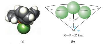
Fig. 23.4 (a) A space-filling diagram of an FePPh<sub>3</sub> unit; the phenyl groups adopt a 'paddle-wheel' arrangement; colour code: Fe, green; P, orange; C, grey; H, white. (b) Schematic representation of the measurement of the Tolman cone angle,  $\theta$ , for a PR<sub>3</sub> ligand; each circle represents the spatial extent of an R group.
