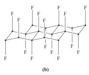
Fig. 13.4 (a) Part of the infinite layered-lattice of  $\alpha$ -graphite ('normal' graphite); the layers are co-parallel, and atoms in *alternate* layers lie over each other. This is emphasized by the yellow lines in the diagram. (b) Part of one layer of the structure of  $CF_n$  for n = 1.
