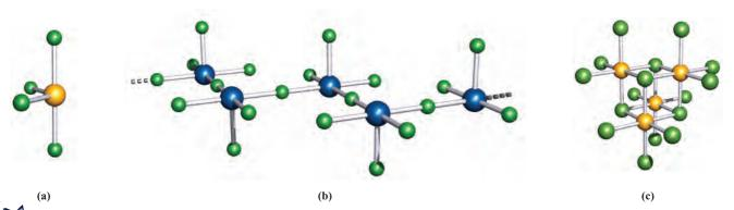
Fig. 15.13 (a) The structure of SeF<sub>4</sub> in the gas and liquid phases; (b) in the solid state, TeF<sub>4</sub> consists of polymeric chains; (c) the structure of the molecular Se<sub>4</sub>Cl<sub>16</sub>-unit present in the crystal lattice of SeCl<sub>4</sub>. Colour code: Se, yellow; Te, blue; F and Cl, green.
