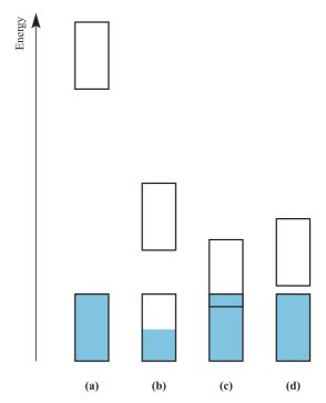
**Fig. 5.12** The relative energies of occupied and empty bands in (a) an insulator, (b) a metal in which the lower band is only *partially* occupied, (c) a metal in which the occupied and empty bands overlap, and (d) a semiconductor.
