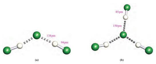
Fig. 8.4 The structures of the anions (a)  $[H_2F_3]^-$  and (b)  $[H_3F_4]^-$ , determined by low-temperature X-ray diffraction for the  $[Me_4N]^+$  salts. The distances given are the average values for like internuclear separations; the experimental error on each distance is  $\pm 3$ –6 pm [D. Mootz et al. (1987) Z. Anorg. Allg. Chem., vol. 544, p. 159]. Colour code: F, green; H, white.
