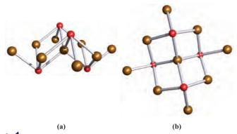
Fig. 13.25 Two views (a) from the side and (b) from above of a part of one layer of the SnO and red PbO lattices. Colour code: Sn, Pb, brown; O, red.
