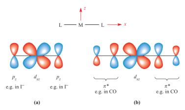
Fig. 20.13  $\pi$ -Bond formation in a linear L-M-L unit in which the metal and ligand donor atoms lie on the x axis: (a) between metal  $d_{xz}$  and ligand  $p_z$  orbitals as for L =  $I^-$ , an example of a  $\pi$ -donor ligand; and (b) between metal  $d_{xz}$  and ligand  $\pi^*$ -orbitals as for L = CO, an example of a  $\pi$ -acceptor ligand.
