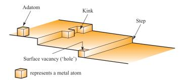
**Fig. 26.11** A schematic representation of typical features of a metal surface. [Based on a figure from *Encyclopedia of Inorganic Chemistry* (1994), R. B. King (ed.), vol. 3, p. 1359, John Wiley & Sons: Chichester.]
