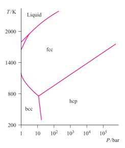
Fig. 5.7 A pressure–temperature phase diagram for iron.
