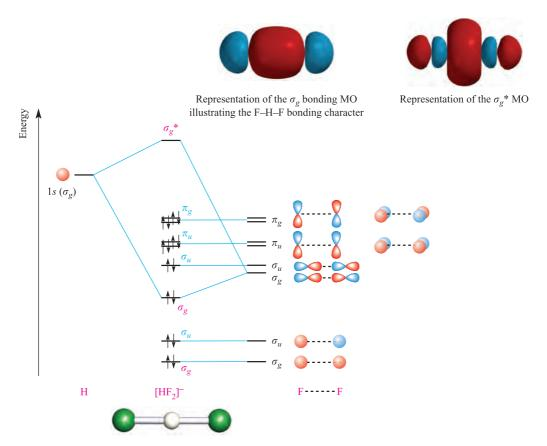
Fig. 4.29 A qualitative MO diagram for the formation of  $[HF_2]^-$  using a ligand group orbital approach. The characters of the  $\sigma_g$  and  $\sigma_g^*$  MOs are shown at the top of the figure.
