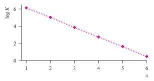
**Fig. 6.11** Stepwise stability constants for the formation of  $[Al(H_2O)_{6-x}F_x]^{(3-x)+}$  (x = 1-6).
