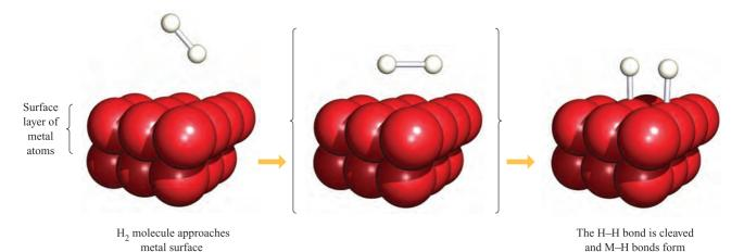
Fig. 9.3 A schematic representation of the interaction of an  $H_2$  molecule with a metal surface to give *adsorbed* hydrogen atoms. The scheme does not imply anything about the detailed mechanism of the process. Further details about heterogeneous catalysis are given in Chapter 26.
