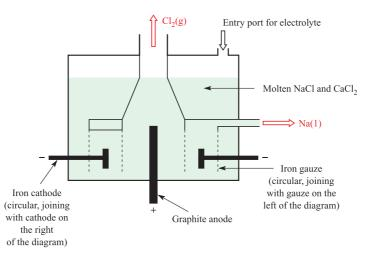
Fig. 10.1 A schematic representation of the electrolysis cell used in the Downs process to produce sodium commercially from NaCl. The products (Na and Cl<sub>2</sub>) must be kept separate from each other to prevent recombination to form NaCl.
