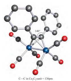
Fig. 23.19 The structure (X-ray diffraction) of  $Co_2(CO)_6(C_2Ph_2)$  [D. Gregson *et al.* (1983) *Acta Crystallogr.*, *Sect. C*, vol. 39, p. 1024]. Hydrogen atoms are omitted for clarity; colour code: Co, blue; C, grey; O, red.
