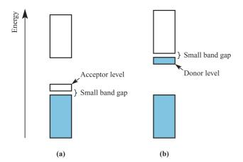
**Fig. 5.13** (a) In a p-type semiconductor (e.g. Ga-doped Si), electrical conductivity arises from thermal population of an acceptor level which leaves vacancies (positive holes) in the lower band. (b) In an n-type semiconductor (e.g. As-doped Si), a donor level is close in energy to the conduction band.
