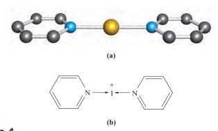
Fig. 16.4 (a) The structure of  $[I(py)_2]^+$  (determined by X-ray crystallography) from the salt  $[I(py)_2][I_3] \cdot 2I_2$  [O. Hassel *et al.* (1961) *Acta Chem. Scand.*, vol. 15, p. 407]; (b) A representation of the bonding in the cation. Colour code: I, gold; N, blue; C, grey.
