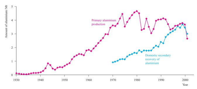
Fig. 12.2 Production of primary aluminium in the US between 1930 and 2001 has risen dramatically; the contribution that recycled aluminium has made to the market became increasingly important in the latter part of the twentieth century and competes with primary production. The term 'secondary aluminium' refers to metal recovered from new and old scrap, and the total production is the sum of primary and secondary sources. [Data: US Geological Survey.]
