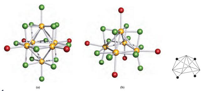
Fig. 22.4 The structures (determined by X-ray diffraction) of (a)  $[Zr_6Cl_{14}(P^nPr_3)_4]$  [F.A. Cotton *et al.* (1992) *Angew. Chem.*, *Int. Ed. Engl.*, vol. 31, p. 1050] and (b)  $[Zr_5Cl_{12}(\mu-H)_2(\mu_3-H)_2(PMe_3)_5]$  [F.A. Cotton *et al.* (1994) *J. Am. Chem. Soc.*, vol. 116, p. 4364]. Colour code: Zr, yellow; Cl, green; P, red; Me and <sup>n</sup>Pr groups are omitted. The inset in (b) shows the μ-H and μ<sub>3</sub>-H positions (black dots) with respect to the  $Zr_5$  framework.
