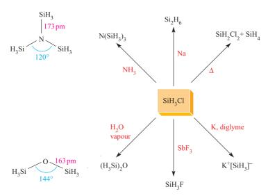
Fig. 13.11 Representative reactions of  $SiH_3Cl$ . The structures of  $N(SiH_3)_3$  (determined by X-ray diffraction at 115 K) and  $(H_3Si)_2O$  (determined by electron diffraction).
