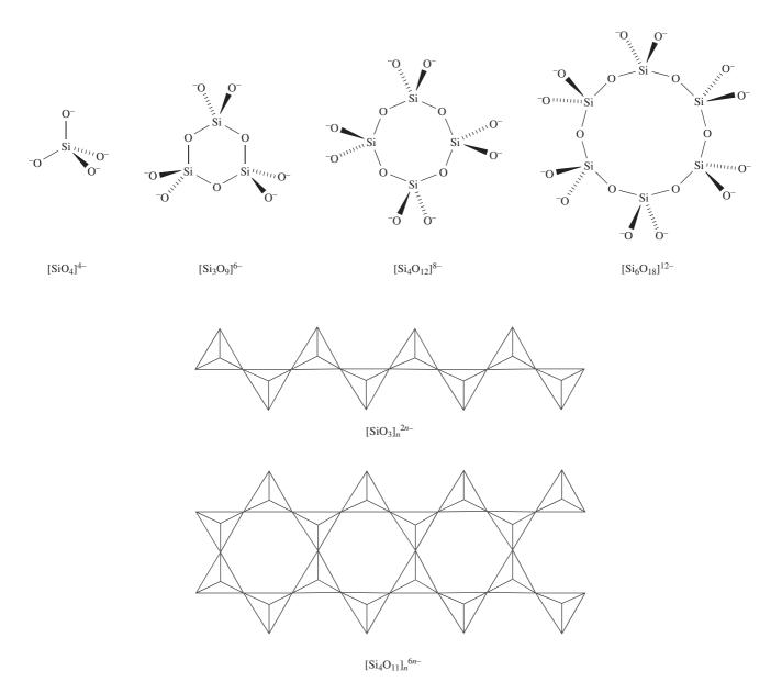
Fig. 13.20 Schematic representations of the structures of selected silicates. Conformational details of the rings are omitted. In the polymeric structures, each tetrahedron represents an SiO<sub>4</sub>-unit as shown in structure 13.17. (See also *Figure 13.22*.)
