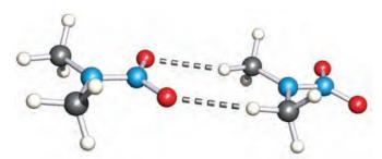
Fig. 9.10 Part of one of the hydrogen-bonded chains in the solid-state structure of Me<sub>2</sub>NNO<sub>2</sub> determined by neutron diffraction [A. Filhol *et al.* (1980) *Acta Crystallogr.*, *Sect. B*, vol. 36, p. 575]. Colour code: C, grey; N, blue; O, red; H, white.
