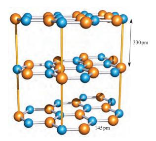
**Fig. 12.18** Part of the layer structure of the common polymorph of boron nitride, BN. Hexagonal rings in adjacent layers lie over one another so that B and N atoms are eclipsed. This is emphasized by the yellow lines.
