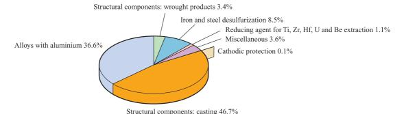
Fig. 11.2 Uses of Mg in the US in 2001 [data from US Geological Survey]; for a discussion of cathodic protection, see Box 7.3.
