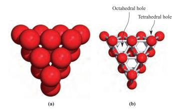
**Fig. 5.5** Two layers of close-packed atoms shown (a) with the spheres touching, and (b) with the sizes of the spheres reduced so that connectivity lines are visible. In (b), the tetrahedral and octahedral holes are indicated.
