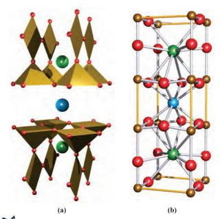
Fig. 27.6 A unit cell of YBa<sub>2</sub>Cu<sub>3</sub>O<sub>7</sub>. (a) A representation showing coordination polyhedra for the Cu centres (square planar and square-based pyramidal); the Y<sup>3+</sup> and Ba<sup>2+</sup> ions are shown in blue and green respectively. (b) The unit cell drawn using a 'ball-and-stick' representation; colour code: Cu, brown; Y, blue; Ba, green; O, red.
