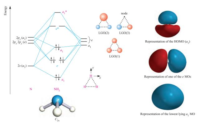
Fig. 4.19 A qualitative MO diagram for the formation of NH<sub>3</sub> using the ligand group orbital approach. For clarity, the lines marking degenerate orbital energies are drawn apart. The diagrams on the right-hand side show representations of three of the occupied MOs; the orientation of the NH<sub>3</sub> molecule in each diagram is the same as in the structure at the bottom of the figure.
