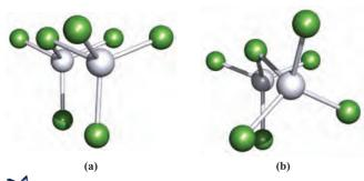
Fig. 8.7 The crystallographically determined structure of the [Al<sub>2</sub>Cl<sub>7</sub>]<sup>-</sup> ion. In the compound [(C<sub>6</sub>Me<sub>6</sub>)<sub>3</sub>Zr<sub>3</sub>Cl<sub>6</sub>][Al<sub>2</sub>Cl<sub>7</sub>]<sub>2</sub>, the anions adopt one of two different conformations: (a) an eclipsed conformation and (b) a staggered conformation [F. Stollmaier *et al.* (1981) *J. Organomet. Chem.*, vol. 208, p. 327]. Colour code: Al, grey; Cl, green.
