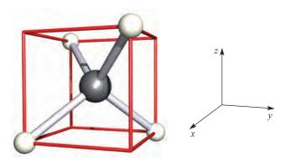
Fig. 20.7 The relationship between a tetrahedral  $ML_4$  complex and a cube; the cube is readily related to a Cartesian axis set. The ligands lie *between* the x, y and z axes; compare this with an octahedral complex, where the ligands lie on the axes.
