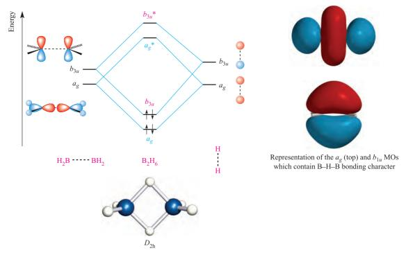
Fig. 4.33 A qualitative, partial MO diagram showing the formation of the B-H-B bridging interactions. The B-H and B-H-B bonding character of the  $a_g$  MO, and the B-H-B bonding character of the  $b_{3u}$  MO are shown in the diagrams on the right-hand side; the orientation of the molecule is the same as in the structure at the bottom of the figure.
