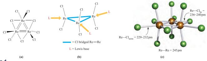
Fig. 22.13 Schematic representations of (a) the structure of Re<sub>3</sub>Cl<sub>9</sub> (interactions between units occur in the solid, see text) and (b) the sites of addition of Lewis bases to Re<sub>3</sub>Cl<sub>9</sub>. (c) The structure (X-ray diffraction) of [Re<sub>3</sub>Cl<sub>12</sub>]<sup>3-</sup> in the [Me<sub>3</sub>NH]<sup>+</sup> salt [M. Irmler *et al.* (1991) Z. Anorg. Allg. Chem., vol. 604, p. 17]; colour code: Re, brown; Cl, green.
