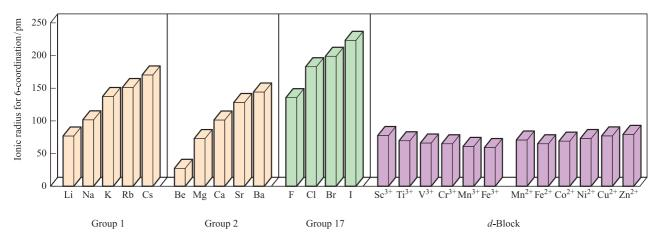
Fig. 5.14 Trends in ionic radii,  $r_{ion}$ , within the metal ions of groups 1 and 2, the anions of group 17, and metal ions from the first row of the d-block.
