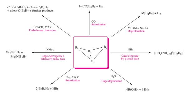
Fig. 12.26 Selected reactions of the arachno-borane B<sub>4</sub>H<sub>10</sub>; the numbering scheme in the central structure is used to denote positions of substitution in products that retain the B<sub>4</sub>-core.
