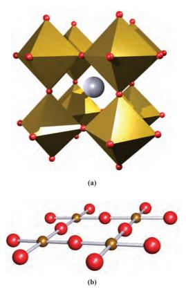
Fig. 27.5 (a) A unit cell of perovskite, CaTiO<sub>3</sub>, using a polyhedral representation for the coordination environments of the Ti centres; an O atom (red) lies at each vertex of the octahedra, and the Ca<sup>2+</sup> ion is shown in grey. (b) Part of a layer of stoichiometry CuO<sub>2</sub> which forms a building block in all cuprate high-temperature superconductors; colour code: Cu, brown; O, red.
