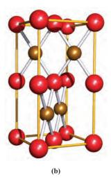
Fig. 21.29 (a) Representation of the solid state structure of CuCl<sub>2</sub> in which chains stack to place each Cu(II) centre in a distorted octahedral environment; (b) the *cooperite* (PtS) structure adopted by CuO with Cu<sup>2+</sup> (square planar) and O<sup>2-</sup> (distorted tetrahedral) centres shown in brown and red respectively. The edges of the unit cell are defined by the vellow lines.
