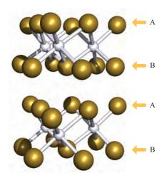
Fig. 5.22 Parts of two layers of the CdI<sub>2</sub> lattice; Cd<sup>2+</sup> ions are shown in pale grey and I<sup>-</sup> ions in gold. The I<sup>-</sup> ions are arranged in an hcp array.
