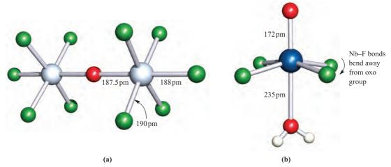
Fig. 22.5 The structures (determined by X-ray diffraction for the  $[Et_4N]^+$  salts) of (a)  $[Ta_2OF_{10}]^{2-}$  [J.C. Dewan *et al.* (1977) *J. Chem. Soc., Dalton Trans.*, p. 978] and (b)  $[Nb(H_2O)(O)F_4]^-$  [N.G. Furmanova *et al.* (1992) *Kristallografiya*, vol. 37, p. 136]. Colour code: Ta, pale grey; Nb, blue; F, green; O, red; H, white.
