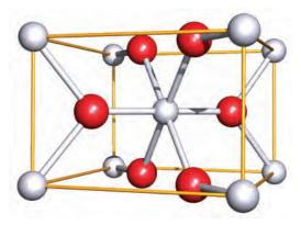
Fig. 5.21 The unit cell of rutile (one polymorph of TiO<sub>2</sub>); the titanium centres are shown in grey and the oxygen centres in red.
