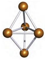
Fig. 8.3 The Zintl ion  $[Sn_5]^{2-}$  has a trigonal bipyramidal cluster structure.
