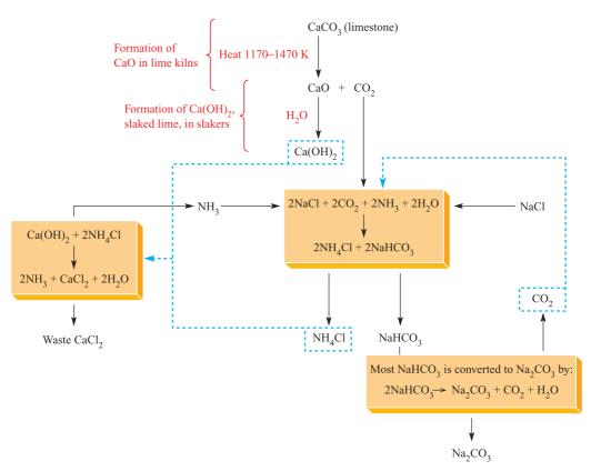
Fig. 10.5 Schematic representation of the Solvay process for the manufacture of Na<sub>2</sub>CO<sub>3</sub> and NaHCO<sub>3</sub> from CaCO<sub>3</sub>, NH<sub>3</sub> and NaCl. The recycling parts of the process are shown with blue, broken lines.
