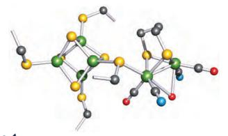
Fig. 28.17 The structure of the hydrogen cluster in the Fe-only hydrogenase from *Desulfovibrio desulficans*. The  $Fe_4S_4$ -cluster has four associated Cys residues, one of which bridges to the  $Fe_2S_2$ -unit. The right-hand Fe atom is coordinatively unsaturated (see text). Colour code: Fe, green; S, yellow; C, grey; N, blue; O, red. Each non-terminated stick represents the connection of a coordinated amino acid to the protein backbone.
