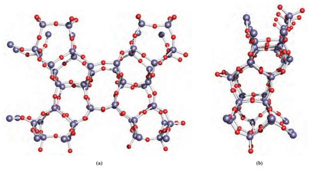
Fig. 13.23 The structure of H-ZSM-5 zeolite (Al<sub>0.08</sub>Si<sub>23.92</sub>O<sub>48</sub>) is typical of a zeolite in possessing cavities which can accommodate guest molecules. (a) and (b) show two orthogonal views of the host lattice; the structure was determined by X-ray diffraction for the zeolite hosting 1,4-dichlorobenzene [H. van Koningsveld *et al.* (1996) *Acta Crystallogr.*, *Sect. B*, vol. 52, p. 140]. Colour code: (Si, Al), purple; O, red.
