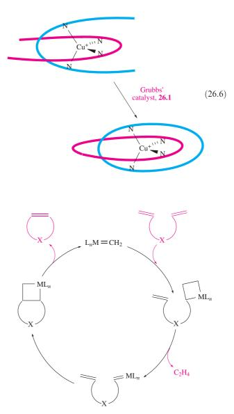
Fig. 26.4 A catalyic cycle for ring-closure metathesis (RCM) showing the Chauvin mechanism which involves [2+2]-cycloadditions and cycloreversions.
