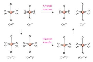
**Fig. 25.9** The outer-sphere mechanism: when the reactants have differing bond lengths, vibrationally excited states with equal bond lengths must be formed in order to allow electron transfer to occur.
