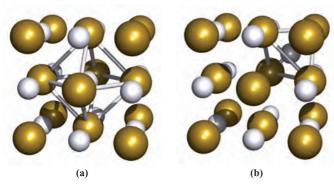
**Fig. 5.27** Silver bromide adopts an NaCl lattice. (a) An ideal lattice can be described in terms of Ag<sup>+</sup> ions occupying octahedral holes in a cubic close-packed array of bromide ions. (b) A Frenkel defect in AgBr involves the migration of Ag<sup>+</sup> ions into tetrahedral holes; in the diagram, one Ag<sup>+</sup> ion occupies a tetrahedral hole which was originally vacant in (a), leaving the central octahedral hole empty. Colour code: Ag, pale grey; Br, gold.
