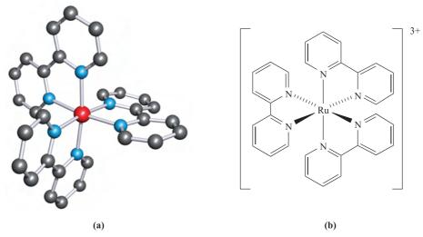
Fig. 9.2 (a) The structure of  $[Ru(bpy)_3]^{3+}$  (bpy = 2,2'-bipyridine) determined by X-ray diffraction for the compound  $[Ru(bpy)_3][PF_6]_3$  [M. Biner *et al.* (1992) *J. Am. Chem. Soc.*, vol. 114, p. 5197], and (b) a schematic representation of  $[Ru(bpy)_3]^{3+}$ . Colour code: Ru, red; C, grey; N, blue; H atoms are omitted.
