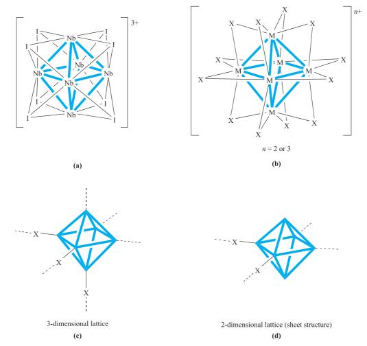
Fig. 22.6 Representations of the structures of (a) the  $[Nb_6I_8]^{3+}$  unit found in  $Nb_6I_{11}$  and (b) the  $[M_6X_{12}]^{n+}$  (n=2 or 3) unit found in compounds of type  $M_6X_{14}$  and  $M_6X_{15}$  for M=Nb or Ta, X=halide. The cluster units are connected into (c) a 3-dimensional network or (d) a 2-dimensional sheet by bridging halides (see text).
