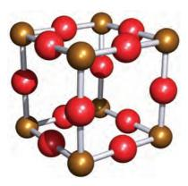
Fig. 21.4 Unit cell of ReO<sub>3</sub>; Re atoms are shown in brown and O atoms in red. This structure type is adopted by ScF<sub>3</sub> and FeF<sub>3</sub>.
