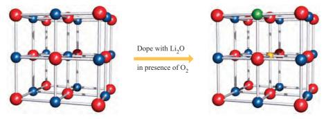
Fig. 27.1 NiO possesses an NaCl structure; doping with Li<sub>2</sub>O in the presence of air/O<sub>2</sub> results in the replacement of an Ni<sup>2+</sup> centre (blue) with an Li<sup>+</sup> ion (yellow), and the oxidation of one Ni<sup>2+</sup> to an Ni<sup>3+</sup> centre (green). Oxide ions are shown in red.
