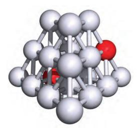
Fig. 5.8 In a substitutional alloy, some of the atom sites in the host lattice (shown in grey) are occupied by solute atoms (shown in red).
