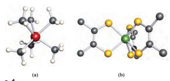
Fig. 19.6 The trigonal prismatic structures of (a) [WMe<sub>6</sub>] [V. Pfennig *et al.* (1996) *Science*, vol. 271, p. 626] and (b) [Re(S<sub>2</sub>C<sub>2</sub>Ph<sub>2</sub>)<sub>3</sub>], only the *ipso*-C atoms of each Ph ring are shown [R. Eisenberg *et al.* (1966) *Inorg. Chem.*, vol. 5, p. 411]. Hydrogen atoms are omitted from (b); colour code: W, red; Re, green; C, grey; S, yellow; H, white.
