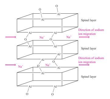
Fig. 27.2 A schematic representation of part of the structure of β-alumina (Na<sub>2</sub>O·11Al<sub>2</sub>O<sub>3</sub>) in which Na<sup>+</sup> ions are mobile between bridged layers of Al<sub>2</sub>O<sub>3</sub> spinel structure. Spinels were introduced in *Box 12.6*.
