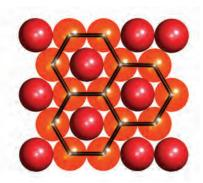
Fig. 5.1 Part of one layer of a close-packed arrangement of equal-sized spheres. It contains hexagonal motifs.
