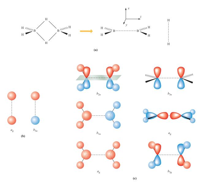
Fig. 4.32 (a) The structure of  $B_2H_6$  can be broken down into  $H_2B_{--}BH_2$  and  $H_{--}H$  fragments. (b) The ligand group orbitals (LGOs) for the  $H_{--}H$  fragment. (c) The six lowest energy LGOs for the  $B_2H_4$  unit; the nodal plane in the  $b_{2u}$  orbital is shown.
