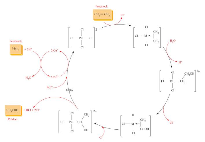
Fig. 26.2 Catalytic cycle for the Wacker process; for simplicity, we have ignored the role of coordinated  $H_2O$ , which replaces  $Cl^-$  trans to the alkene.
