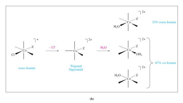
**Fig. 25.7** Octahedral substitution through (a) a square-based pyramidal species leads to retention of the initial *cis*-isomer but through (b), a trigonal bipyramidal species, may lead to isomerization.
