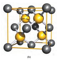
Fig. 5.18 (a) The unit cell of  $CaF_2$ ; the  $Ca^{2+}$  ions are shown in red and the  $F^-$  ions in green. (b) The unit cell of zinc blende (ZnS); the zinc centres are shown in grey and the sulfur centres in yellow. Both sites are equivalent, and the unit cell could be drawn with the  $S^{2-}$  ions in the grey sites.
