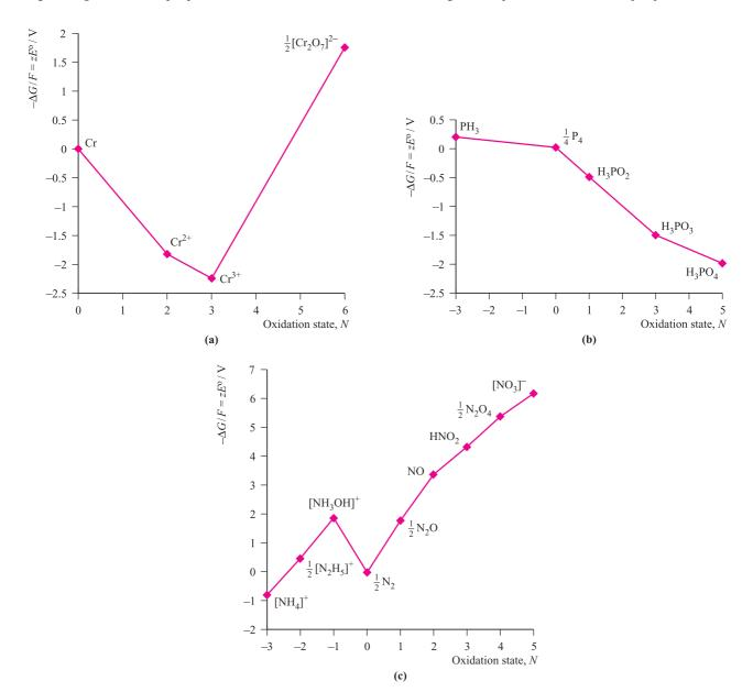
Fig. 7.4 Frost-Ebsworth diagrams in aqueous solution at pH 0, i.e.  $[H^+] = 1 \text{ mol dm}^{-3}$ , for (a) chromium, (b) phosphorus and (c) nitrogen.
