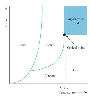
**Fig. 8.8** A simple pressure–temperature phase diagram for a one-component system.
