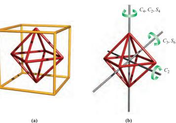
Fig. 4.26 (a) An octahedron can be inscribed in a cube; each vertex of the octahedron lies in the middle of a face of the cube. (b) The diagram shows one of each type of rotation axis of an octahedron. An inversion centre lies at the centre of the octahedron. [*Exercise*: Work out where the  $\sigma_h$  and  $\sigma_d$  planes lie; see Table 4.4.]
