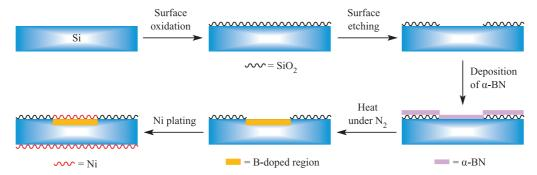
Fig. 27.9 Boron doping of silicon using  $\alpha$ -BN.
