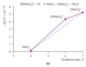
Fig. 7.3 The Frost-Ebsworth diagram for manganese in aqueous solution at pH 0, i.e.  $[H^+] = 1 \text{ mol dm}^{-3}$ .
