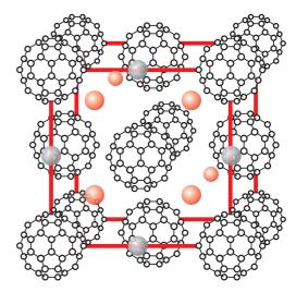
**Fig. 13.9** A representation of the structures of  $K_3C_{60}$  and  $Rb_3C_{60}$  in which the  $[C_{60}]^{3-}$  cages are arranged in an fcc lattice with the  $M^+$  ions occupying all the octahedral (grey) and tetrahedral (red) holes. Some of the cations in the unit cell shown are hidden by  $[C_{60}]^{3-}$  anions.
