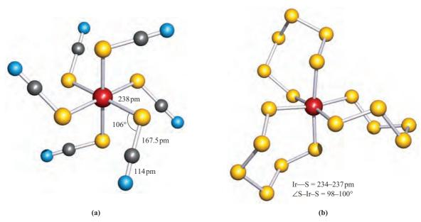
Fig. 22.21 The structures (X-ray diffraction) of (a)  $[Ir(NCS-S)_6]^{3-}$  in the  $[Me_4N]^+$  salt [J.-U. Rohde *et al.* (1998) *Z. Anorg. Allg. Chem.*, vol. 624, p. 1319] and (b)  $[Ir(S_6)_3]^{3-}$  in the  $[NH_4]^+$  salt [T.E. Albrecht-Schmitt *et al.* (1996) *Inorg. Chem.*, vol. 35, p. 7273]. Colour code: Ir, red; S, yellow; C, grey; N, blue.
