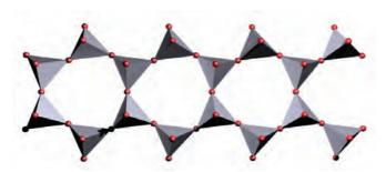
**Fig. 13.22** Part of one of the double chains of general formula  $[Si_4O_{11}]_n^{6n-}$  present in the mineral tremolite. Compare this representation with that in Figure 13.20. Each red sphere represents an O atom, and each tetrahedral  $O_4$ -unit surrounds an Si atom.
