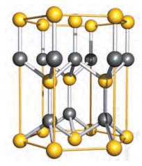
Fig. 5.20 Three unit cells of wurtzite (a second polymorph of ZnS) define a hexagonal prism; the Zn<sup>2+</sup> ions are shown in grey and the S<sup>2-</sup> ions in yellow. Both ions are tetrahedrally sited and an alternative unit cell could be drawn by interchanging the ion positions.
