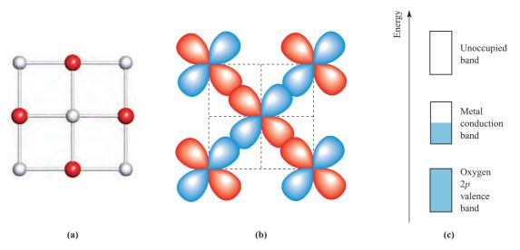
Fig. 27.4 (a) One face of the unit cell of TiO; colour code: Ti, pale grey; O, red. (b) Overlap of the Ti  $t_{2g}$  orbitals occurs and leads to (c) the formation of a partly filled metal conduction band.
