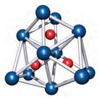
Fig. 10.4 The structure of the suboxide Cs<sub>11</sub>O<sub>3</sub> consists of three oxygen-centred, face-sharing octahedral units. Colour code: Cs, blue; O, red.
