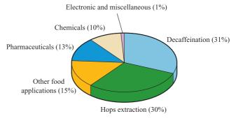
Fig. 8.9 Percentage contributions to the 2001 global US\$960 million value of commercial production using supercritical fluid processing [data: Kline & Company, Inc., www.klinegroup.com].
