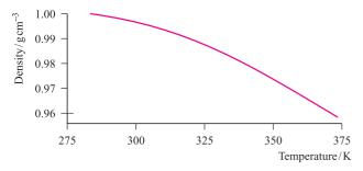
Fig. 6.2 The variation in the value of the density of water between 283 and 373 K.
